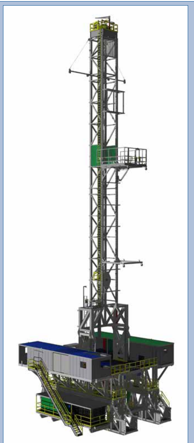
Scandrill Inc.'s first 1,500-hp AC rig, the Scan Vision, is currently working for Anadarko in Loving County, Texas, in the Permian Basin. This Veristic Manufacturing E-Series walking rig's equipment includes OWI 1,600 hp AC drawworks, 3 Caterpillar DGB-3512-C diesel engines with dual-fuel capabilities, a 500 ton Varco TDS-11SA AC top drive, and 2 F-1600 AC drive mud pumps with 7,500 psi fluid ends.
